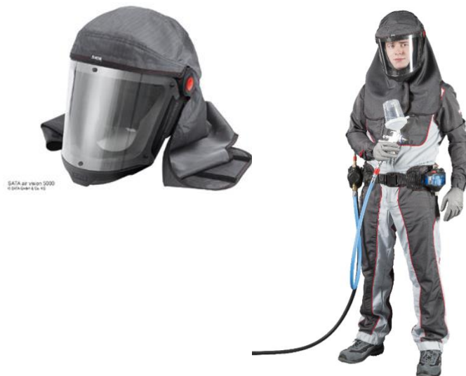
Fig.1.4: left: Hood for a compressed air hose device; right: complete PPE: Compressed air hose device according to EN 14594 class 3 with hood, safety goggles, chemical protection suit (type 5) and gloves. The compressed air hose is connected to the belt and supplies the half-face mask and spray gun with air.
